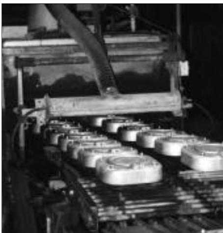
Figure 6. Electric skillets exiting the etch wash before coating and decorating the finished product.
