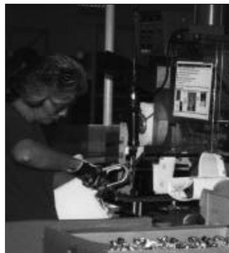
Figure 2. Debbie Kuring performs the job (on an iced tea maker) as described on an operator visual chart. Decorating equipment is used to differentiate various models.
