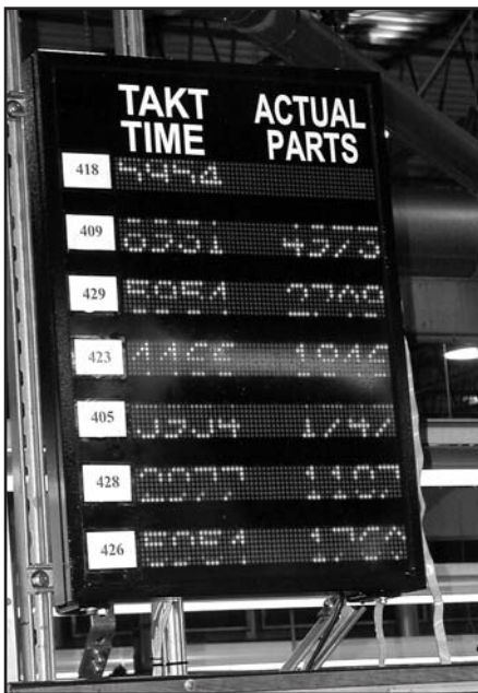
Figure 2. Takt times and other metrics posted in work areas reflect the visual management emphasis at Viking Drill & Tool, Inc.
